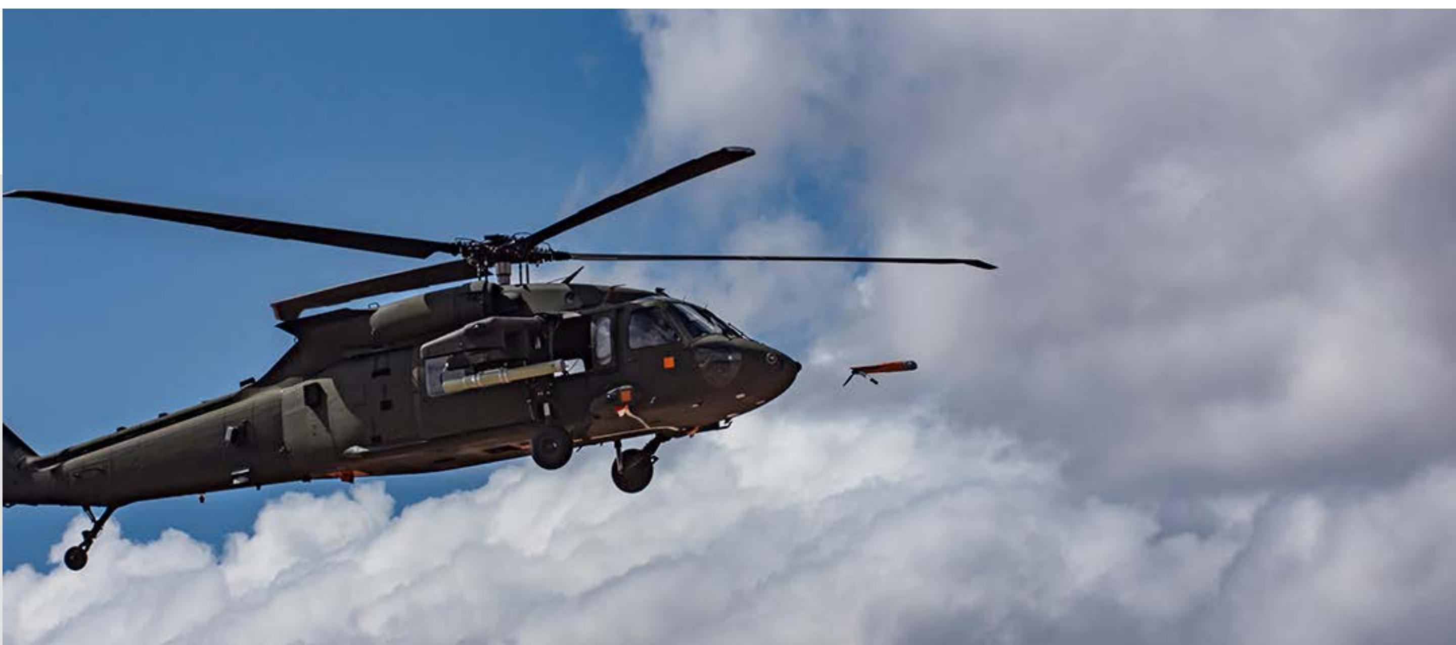
Air Launched Effects Demonstration: Area-I ALTIUS (Agile-Launch, Tactically Integrated, Unmanned System) horizontal launch from a UH-60.
